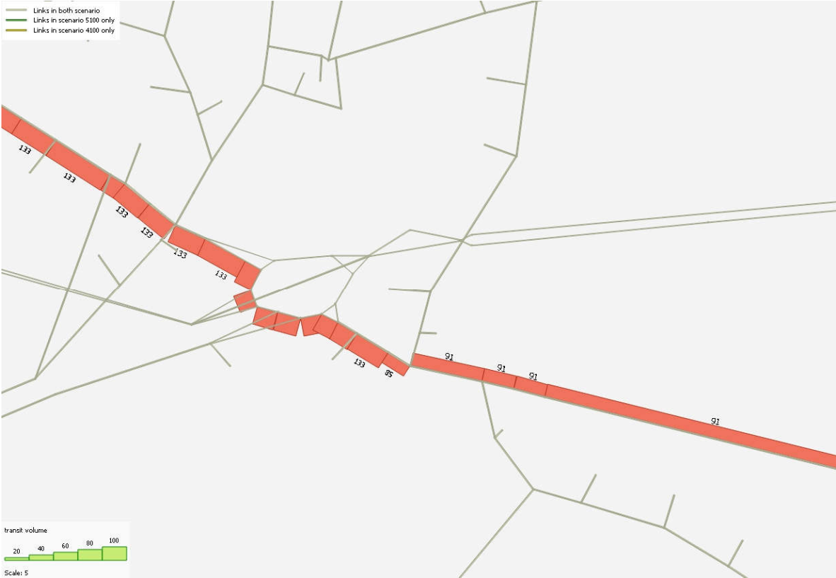
Figure 3-7 - Change in the number of passengers boarding bus services between DM and DS (2021, AM peak hour 08:00 - 09:00)
