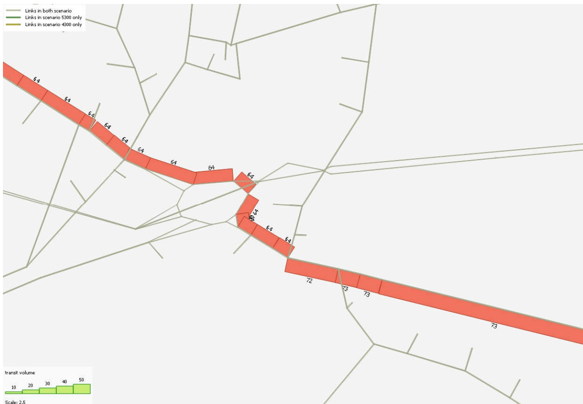
Figure 3-8 Change in the number of passengers boarding bus services between DM and DS (2021, PM peak hour 17:00 - 18:00)
