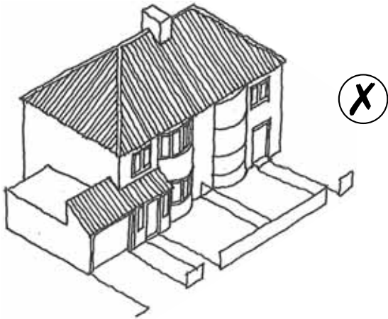
Side extension projecting forwards in front of house Exposed dummy pitch roof
