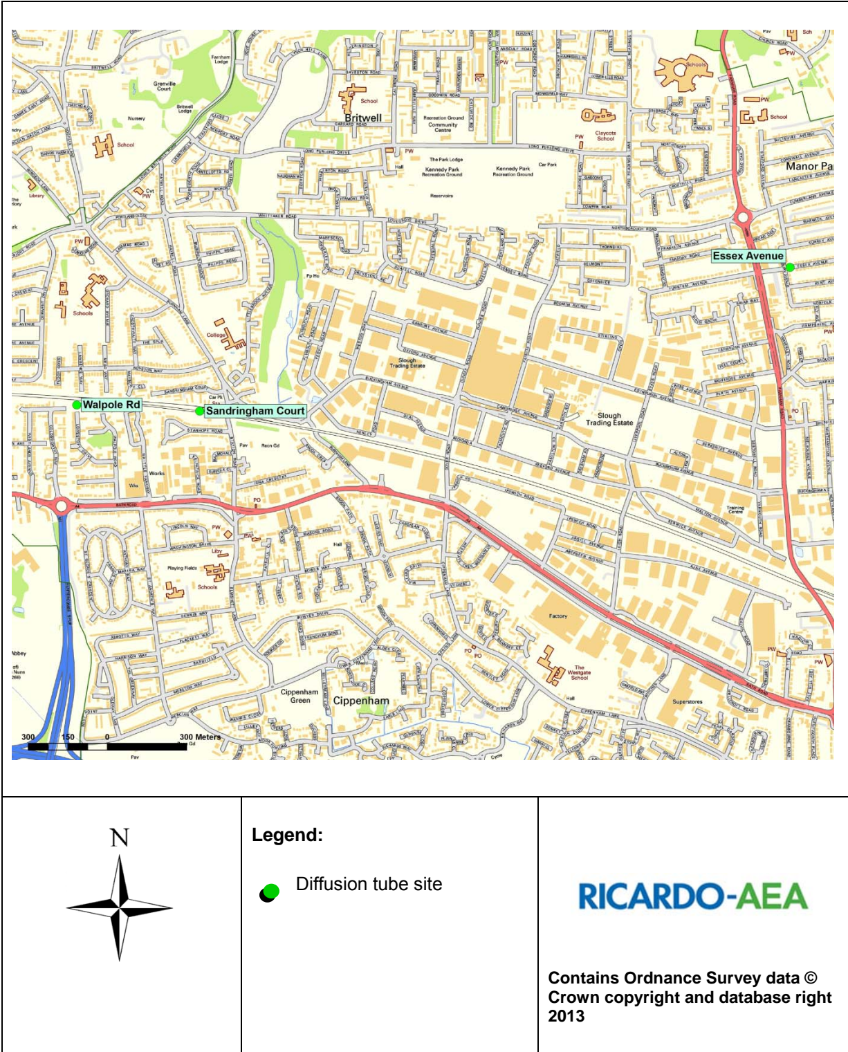
Figure 2.5: Slough diffusion tube locations (Slough North West)
