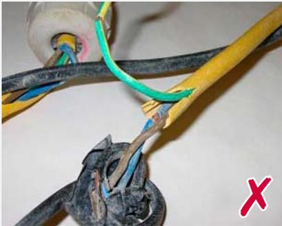
◀ These 240-volt conductors were involved in the death of a builder working on a domestic property. Isolation of supplies, use of earth leakage devices and reduced voltage minimise the risk.
