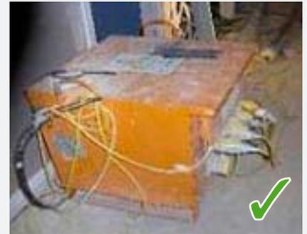
Photograph shows a 110v (centre tapped to earth) electrical supply from a ▲ transformer commonly used on construction sites to reduce the risk of electrocution.
